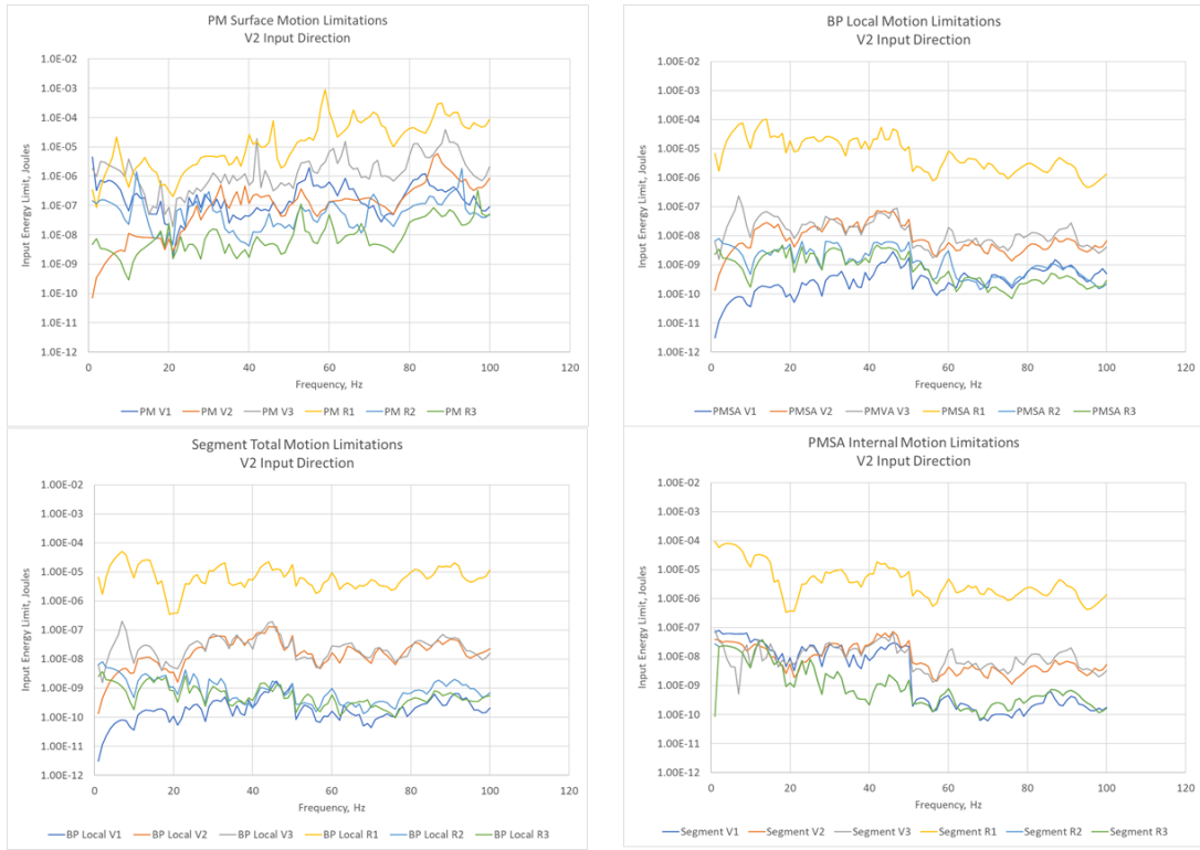
Figure 60: Maximum Energy Limits for V2 disturbance.
